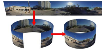
(a) A 360° equirectangular image can be folded over itself until the ends meet.
